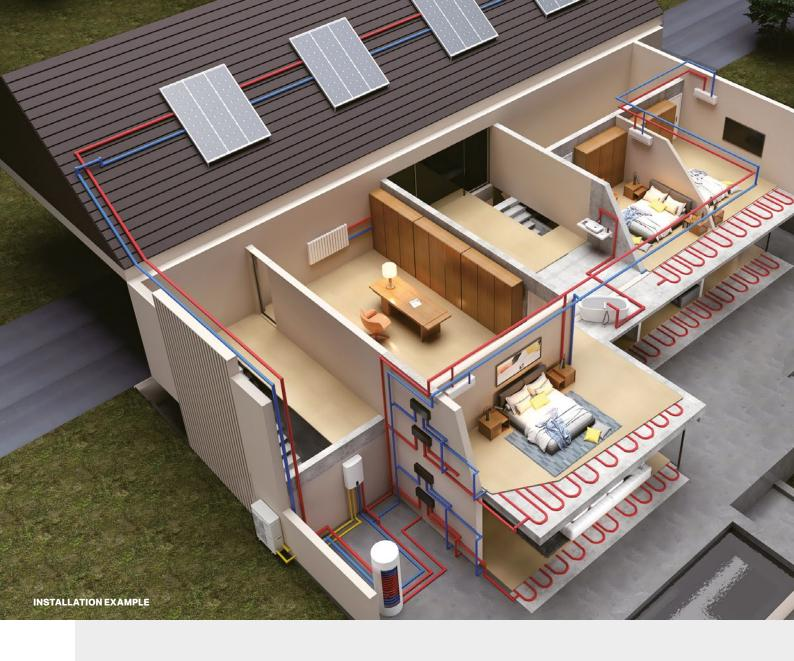
Heat pumps extract free energy from the air and use it to heat or cool the building or prepare domestic hot water. Anyone can benefit from this inexpensive, environmentally friendly and maintenance-free heat source.
